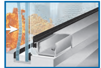
Blast impact shatters external glass and drives it against the inner pane.
